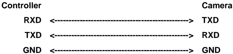
Connection between camera and controller using RS422:
